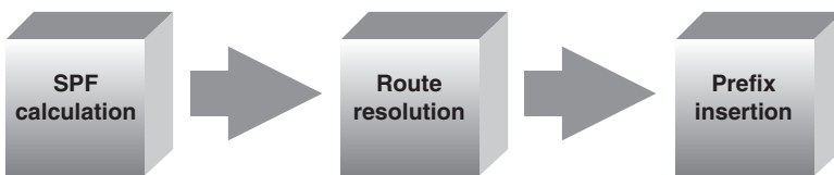
FIGURE 10.1. The three operations for calculating routes
