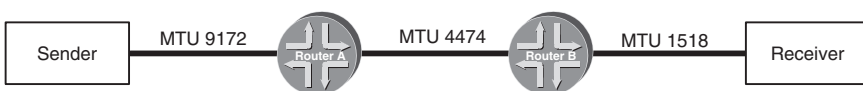
FIGURE 9.2. How does the sender know the MTUs of all the intermediate network segments?
